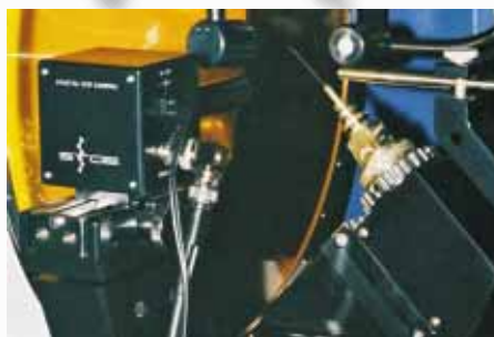
Detailed view of the two-circle goniometer and the video CCD camera.
